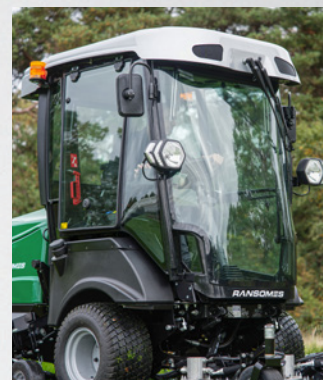
High visibility, spacious operator cabin with SureAir AC & Heater
