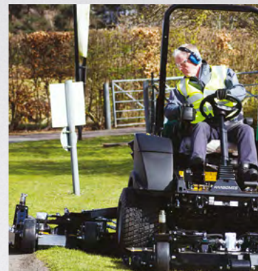
Low maintenance, direct drive hydraulic decks
