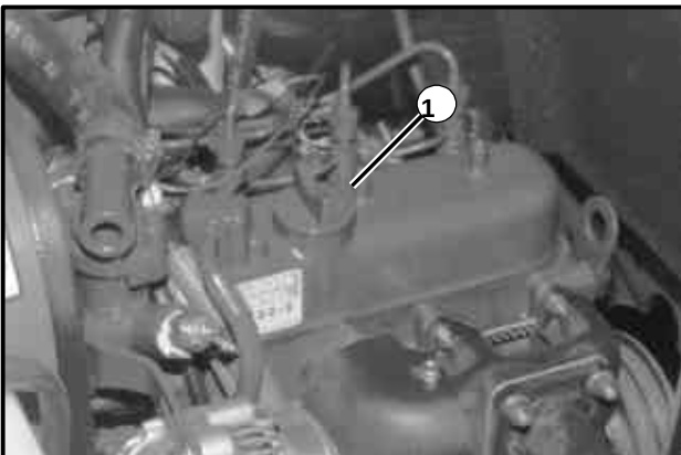
Figuur 27 1. Olie Vulgat (diesel motor)
